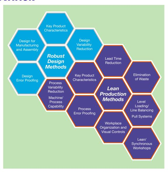
Lean Production methods eliminate inefficiency throughout manufacturing. Special emphasis is placed on operational efficiency that is caused by waste, unevenness, and overburden in manufacturing processes. A collection of methods (as shown in the figure) is used in manufacturing to address this waste. The basic idea is to develop uniform systems that ensure repeatability and consistency of processes.
